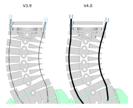
The real cable thickness can be defined in 1D beam elements cable system. In version 4.0 the contact details can be simulated, seatbelt elements cable system doesn't have this advantage behavior.
