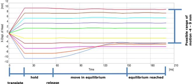
The curves show different phases of Head movement. At the end a possible range of motion is about 4mm forward and 9mm backwards.
