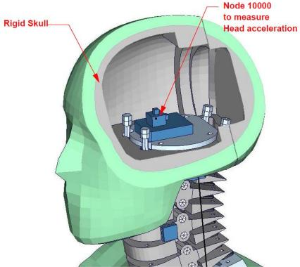
Figure 2: Location of head accelerometer node.
