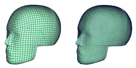
**Figure 12:** Head mesh of v3.5 (left hand side) and v3.8 (right hand side)
