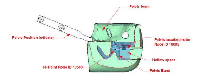
Figure 4: Location of node for extracting pelvis acceleration
