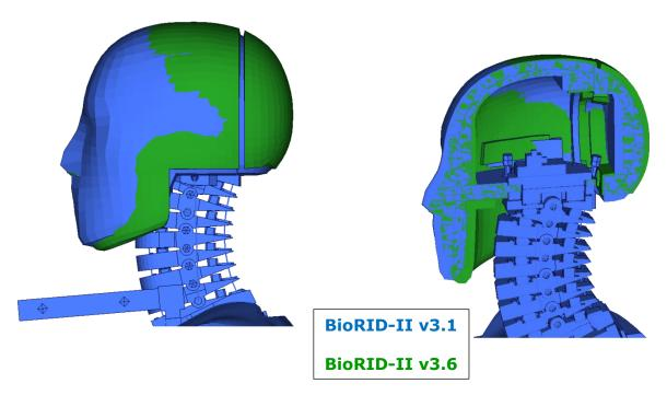
Figure 13: Head geometry of BioRID-II v3.1 compared to v3.6
