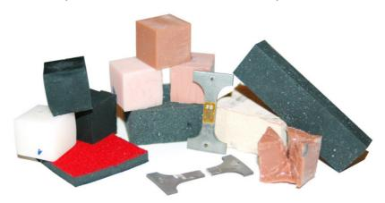
Figure 5: Material test samples of the WorldSID
