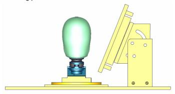
Figure 6: WorldSID head and neck test setup
