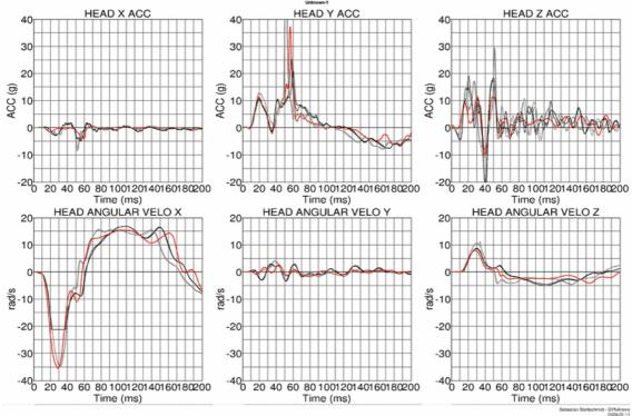
Figure 7: Results of head-neck test, high pulse, 90 degrees
