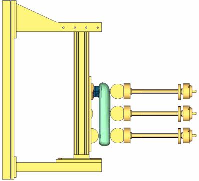
Figure 8: WorldSID arm test setup
