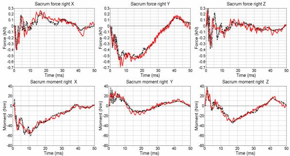
Figure 15: Result of iliac wing test with high velocity, complete pelvis, sacro-iliac load cell
