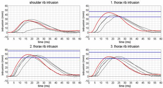
Figure 20: Result of the thorax with half arm calibration test of WSID 50<sup>th</sup> model version 1
