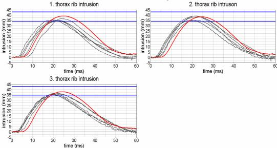
Figure 19: Result of the thorax without arm calibration test of WSID 50<sup>th</sup> model version 1
