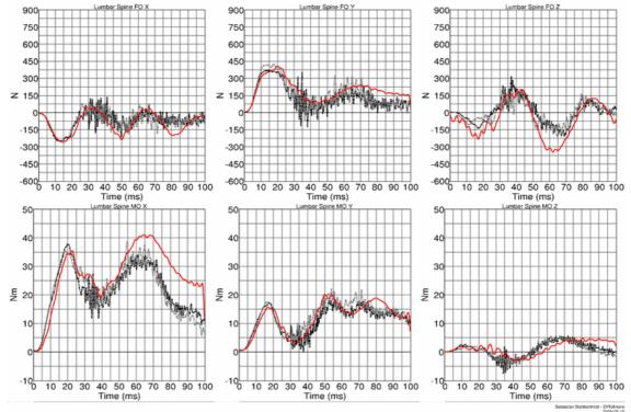
Figure 13: Result of lumbar spine test, lower pulse, 60 degrees lumbar load cell forces and moments
