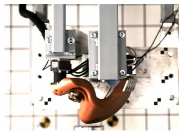
Figure 14: Iliac wing test setup
