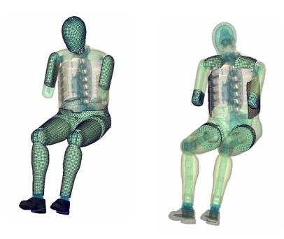
Figure 4: Rubber parts (left) and foam parts (right) of the WorldSID
