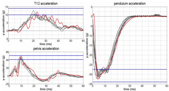
Figure 22: Result of the pelvis calibration test of WSID 50<sup>th</sup> model version 1
