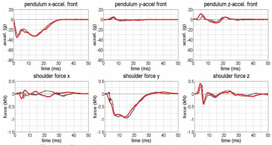
Figure 9: Results of the arm test, middle arm impact, high velocity
