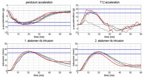
Figure 21: Result of the abdomen calibration test of WSID 50<sup>th</sup> model version 1
