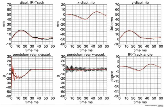
Figure 11: Abdomen rib test on outer band, low velocity and high mass
