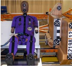
Figure 16: Flat barrier sled test set up with WS50th (left) and barrier with pelvis pusher (right)
