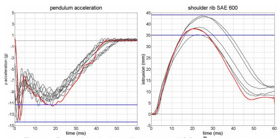
Figure 18: Result of the shoulder calibration test of WSID 50<sup>th</sup> model version 1
