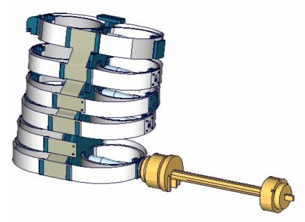
Figure 10: Second abdomen rib test with outer rib band
