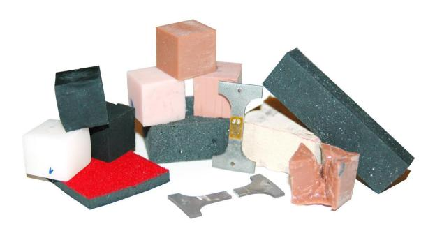
Figure 25: Material test samples of WorldSID
