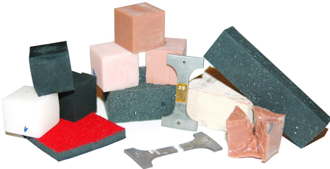
Figure 30: Material test samples of WorldSID
