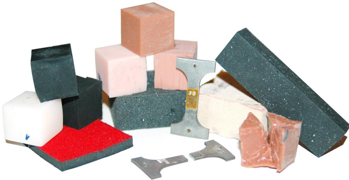
Figure 30: Material test samples of WorldSID
