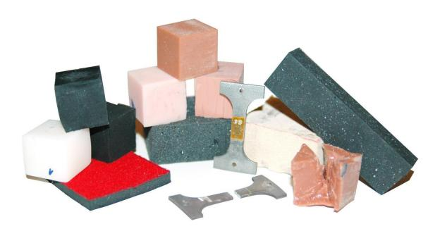
Figure 30: Material test samples of WorldSID
