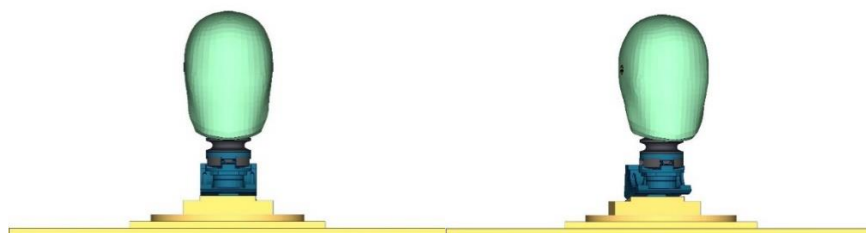
Figure 24: Head neck test setup 90 and 75 degrees
