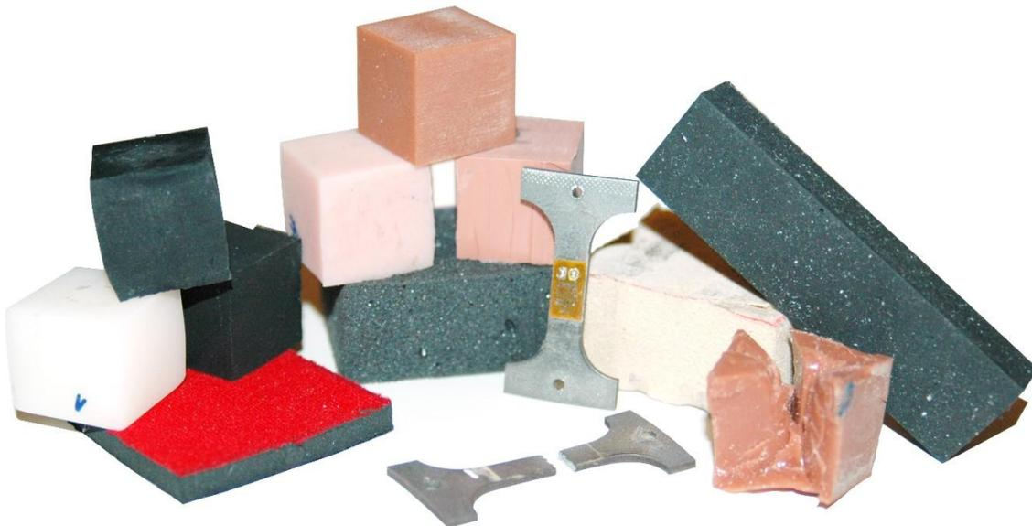
**Figure 19:** Material test samples of WorldSID
