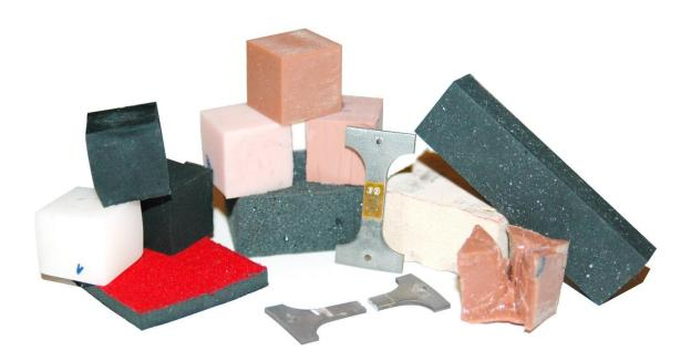
Figure 19: Material test samples of WorldSID
